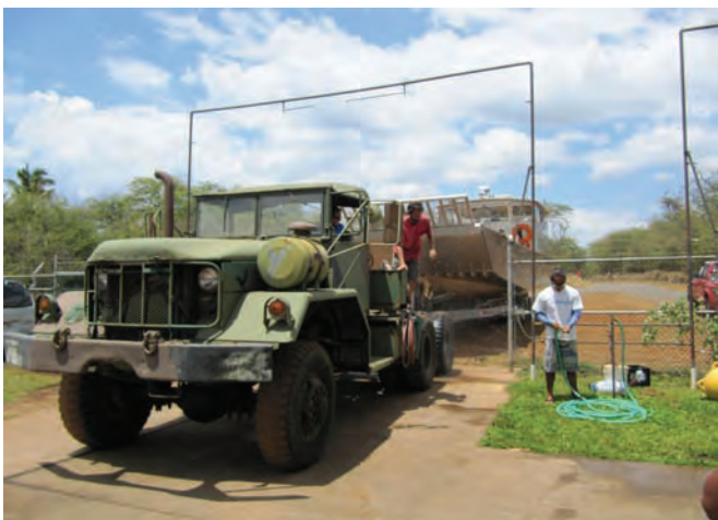
In a constant battle against corrosion, KIRC staff use a fixed boat washing station combined with hand washing to remove salt residue from our equipment.
